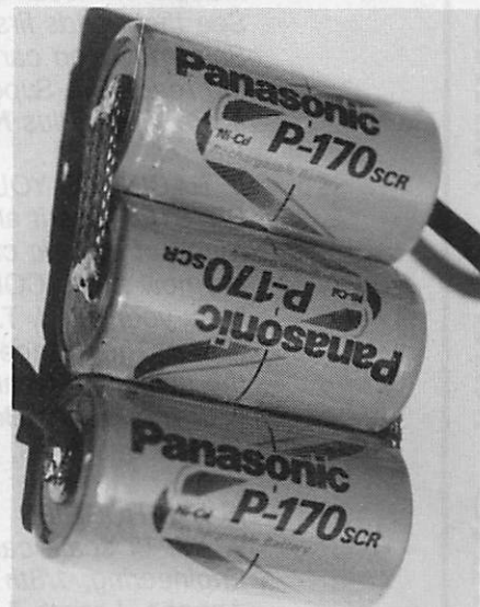
First in the new generation of high capacity, less fragile cells is Panasonics P170 SCR.
